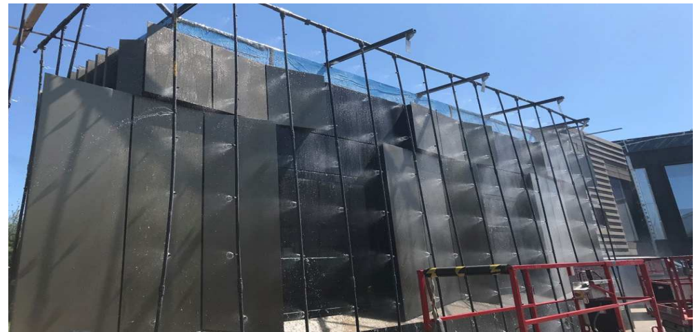
Laboratory air and water testing of full-size facade panels.
