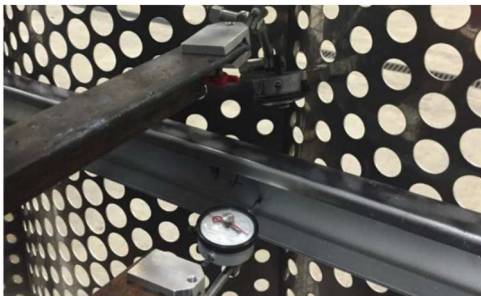
Custom cladding wind testing apparatus
