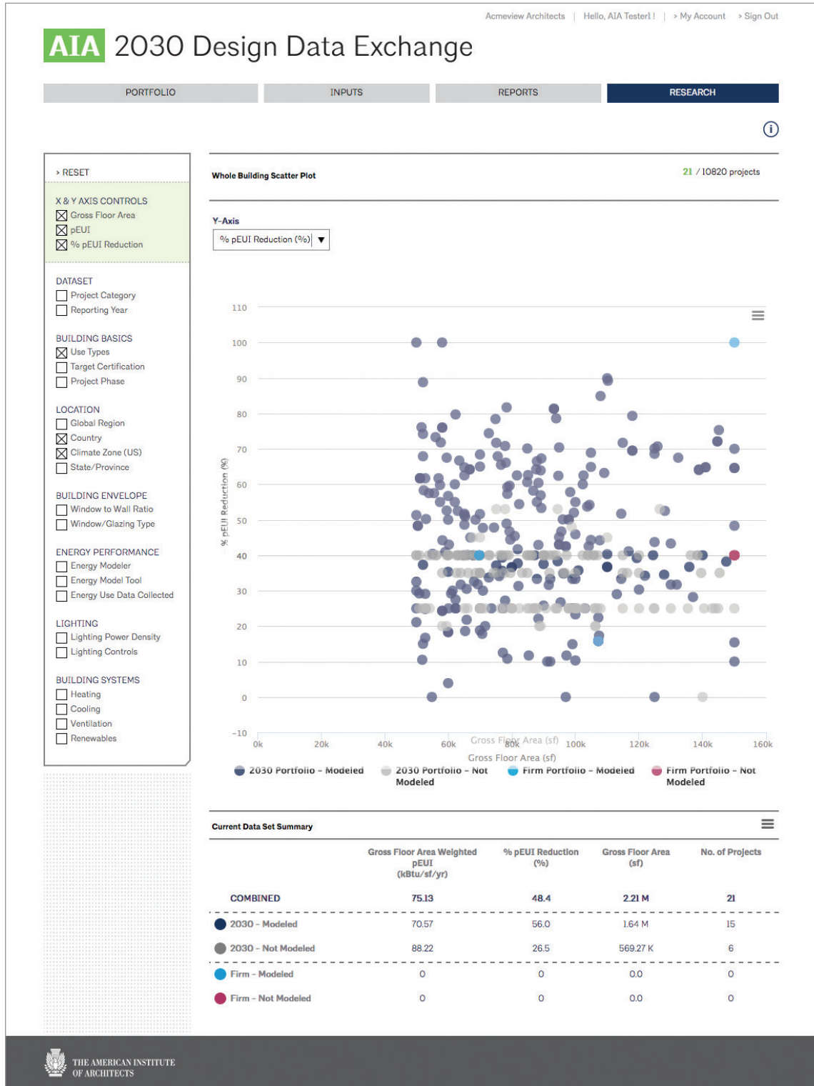
FIGURE 5. Energy benchmarking in the Design Data Exchange
