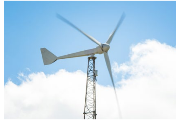
A typical horizontal-axis small wind turbine with blades, rotor, generator/alternator and tail atop a tower.
